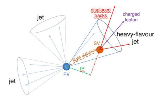
SVX is reconstructed from tracks displaced from the primary vertex
